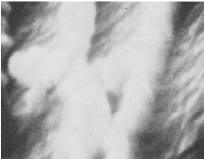
Fig. 19. Scanning electron micrograph of polycarbonate and 7 wt-% butyl rubber blend at high magnification, 1 cm = 0.2 \mu .
